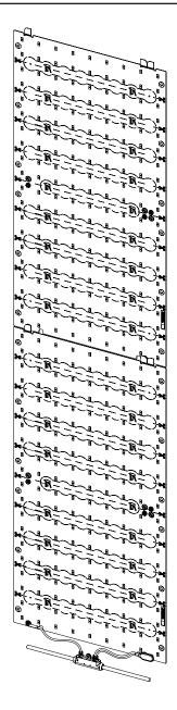
Make the electrical connection between the two (2) TILEs by gently pressing the snap connectors on the overhanging tabs down until they click together.
