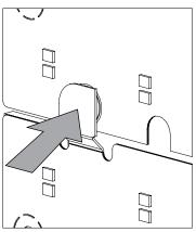
A CAUTION: Disconnecting and reconnecting jumpers may damage the connectors on the sheets if repeated more than 3 times. See Section 7.8 for recommended method.
