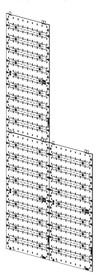
TILEs may not be cut in both directions without breaking the electrical circuits that provide power to the LEDs. For this reason, when installing a run that is <11.8" (300mm) in width, it is necessary to cut the sheets to the required width and then rotate the TILEs 90° so that the input end faces the outer edge of the run. Sheets are cut along the cut line identified in Section 7.2 that corresponds with the required width.
