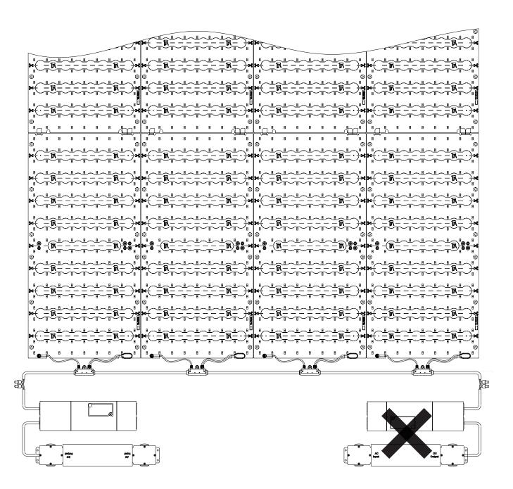
The installation below shows four (4) runs of TILE. Each run consists of two (2) TILE sheets connected in series. The Power Supply or Control Module is connected to the system via the T-Cable and Starter Cable.
