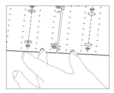
Grip the tab between the thumb and index finger. Gently separate the sheets while keeping the sheets restrained.
