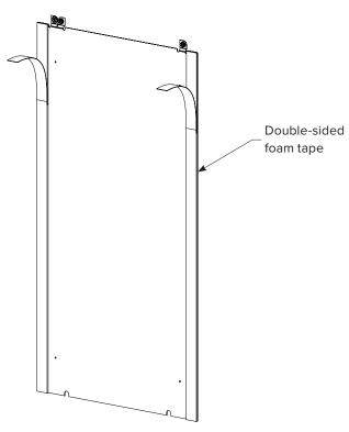
2. Beginning at the input end of a run, position the first TILE where required. Fasten the sheet to the mounting surface using #8 (or M4) fasteners appropriate for the mounting surface. It is recommended to use nylon washers to prevent damage to TILE.
