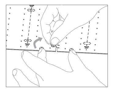
3. Similarly, when disconnecting T-cables from the TILE Interior, the sheet should be restrained while gently separating the connectors.
