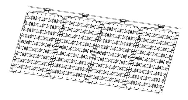
3. T-cables can be cut to length as required. Cutting can be done anywhere on the cables except at the T junctions. After cutting, the end of the cable must be insulated using the T-cable end cap. Slide the end cap over the cable until the cable is fully inserted.
