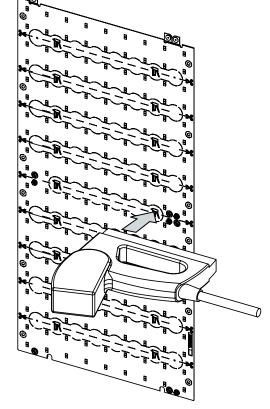
Slide the next TILE under the tabs of the first. Ensure that the flexible tabs on the first TILE sit on top of the second.
